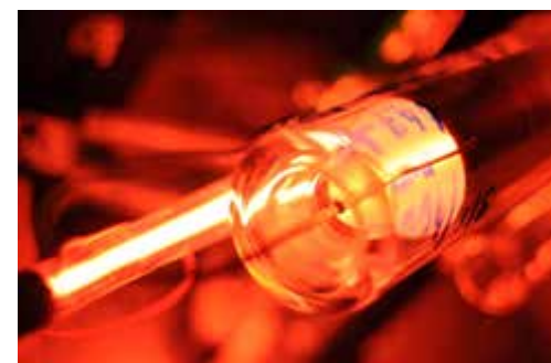
Methane-stabilized HeNe-Laser in a molecular optical clock.
