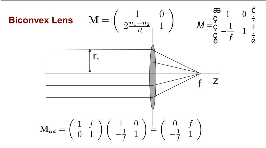
Figure 2.15: Imaging of parallel rays through a lens with focal length f
