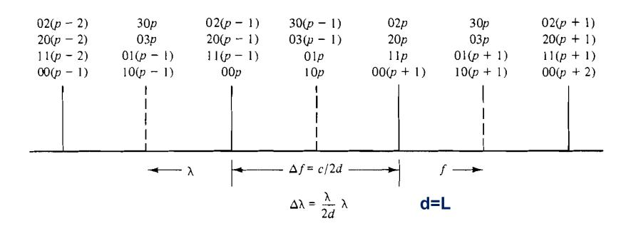
Figure 2.29: Resonance frequencies of the confocal Fabry-Perot resonator,
