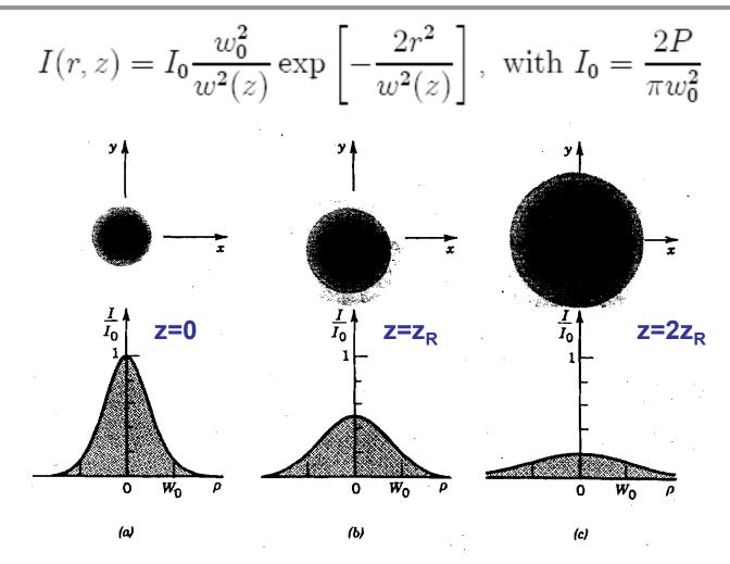
Figure 2.3: The normalized beam intensity  $I/I_0$  as a function of the radial distance r at different axial distances: (a) z=0, (b) z=z<sub>R</sub> (c) z=2z<sub>R</sub>.
