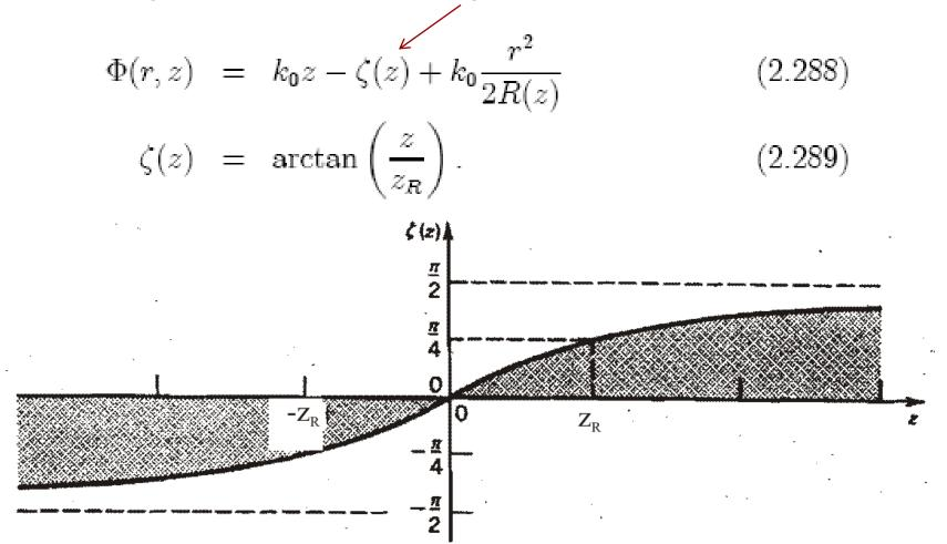
Figure 2.6: Phase delay of Gaussian beam, Guoy-Phase-Shift
