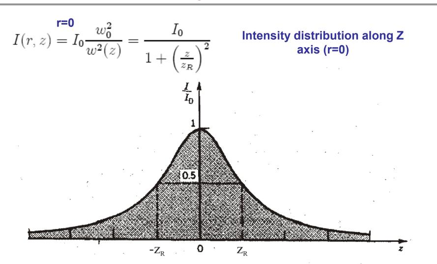
Figure 2.4: Normalized beam intensity I(r=0)/I<sub>0</sub> on the beam axis as a function of propagation distance z.
