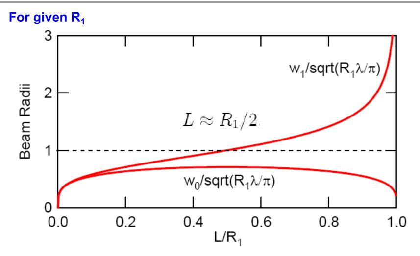
Figure 2.22: Beam waists of the curved-flat mirror resonator as a function of  $L/R_1$ .
