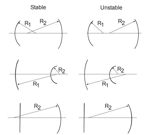
Figure 2.26: Stable and unstable resonators
