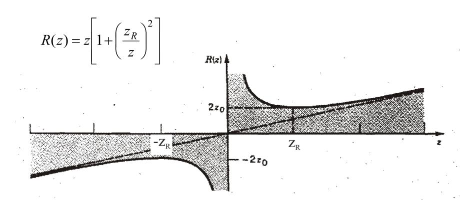
Figure 2.7: Radius of curvature R(z)
