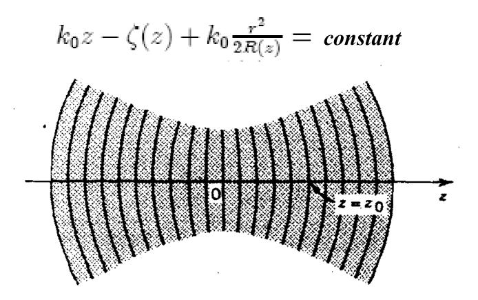
Figure 2.8: Wavefronts of Gaussian beam
