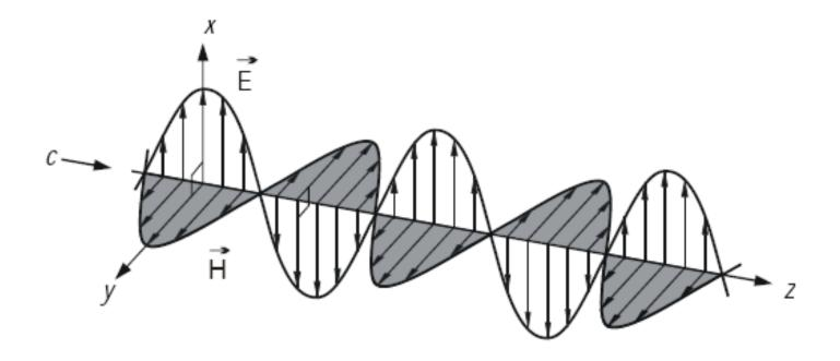
Figure 2.1: Transverse electromagnetic wave (TEM) [6]
