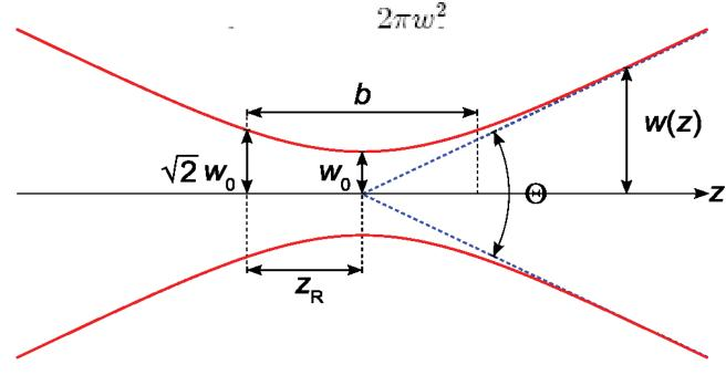
Figure 2.5: Gaussian beam and its characteristics
