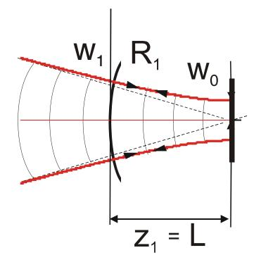
Figure 2.21: Curved-Flat Mirror Resonator  $w_{1} = w_{o} \left[ 1 + \left(\frac{L}{z_{R}}\right)^{2} \right]^{1/2}$ with  $z_{R} = \frac{\pi w_{o}^{2}}{\lambda}$   $R_{1} = L \left[ 1 + \left(\frac{z_{R}}{L}\right)^{2} \right]$   $\sqrt{\lambda R_{1}} \sqrt{L} \left( L + L \right)$
