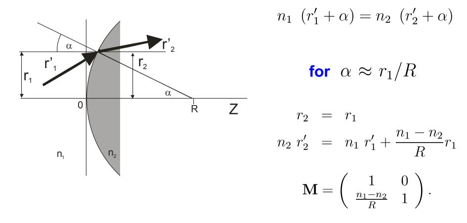
Figure 2.14: Derivation of ABCD-matrix of a thin plano-convex lens.
