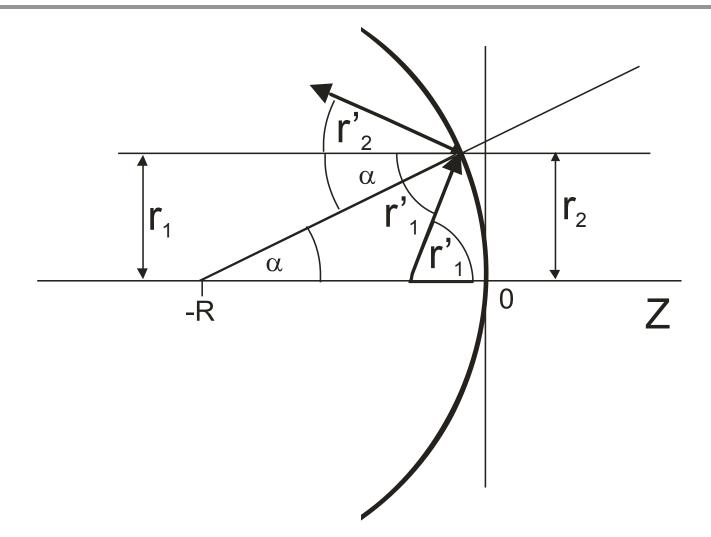
Figure 2.16: Derivation of Ray matrix for concave mirror with Radius R.
