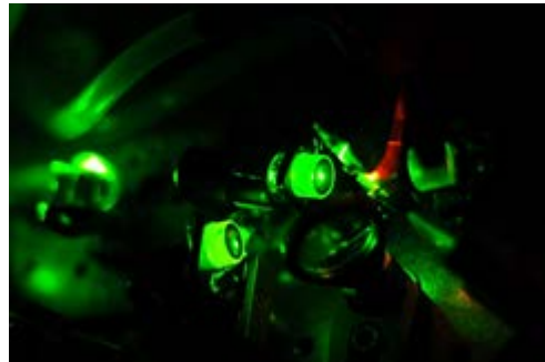
High repetition rate Kerr-Lens Modelocked Ti:sapphire laser
