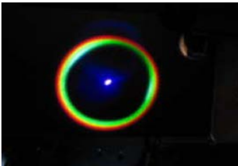
Superfluorescence cone in a parametric amplifier.
