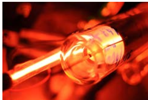
Methan-stabilized HeNe-Laser in a molecular optical clock
