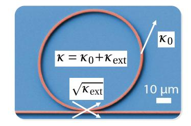
Instead of using resonator eigenmodes to describe system one can use an equidistant frequency grid with frequencies  $\omega_p + \mu D_1$ :
