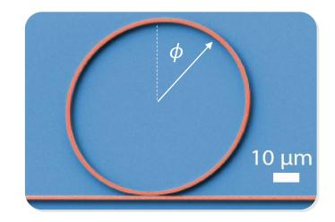
Projection onto mode with index  $\mu$  by multiplication with  $\rho^{-i(\mu\phi-\omega_{\mu}t)}$  and integration over  $\phi$ .
