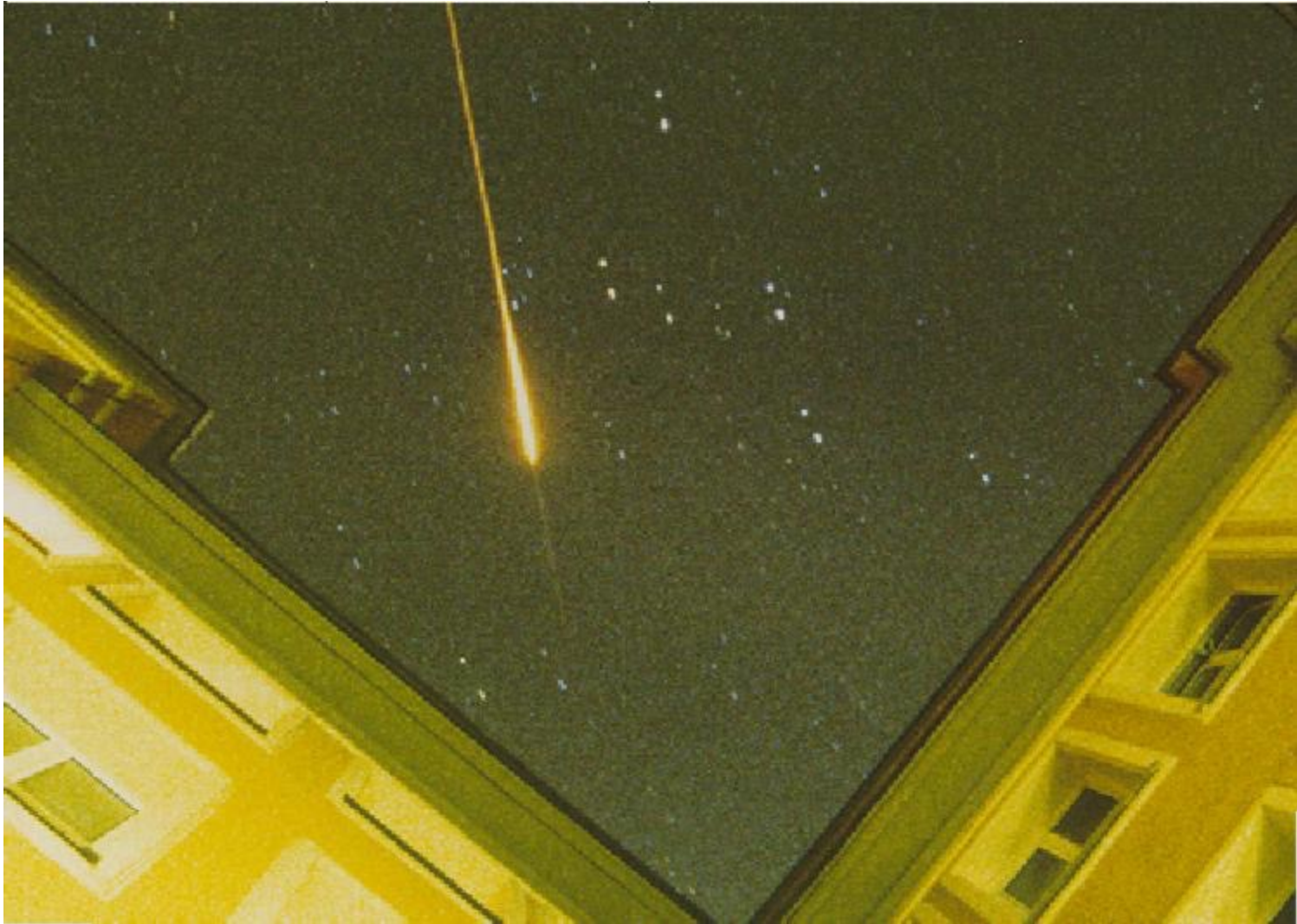
Photograph of a self-guided filament induced in air by a high-power infrared (800 nm) laser pulse [from http://www.teramobile.org ]
