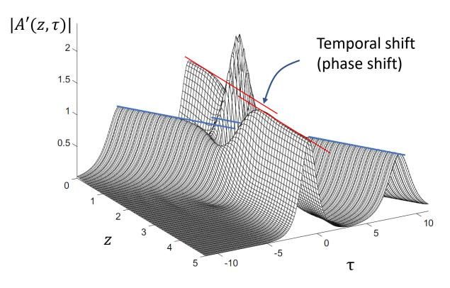
Solitons recover after collision with small phase shift
