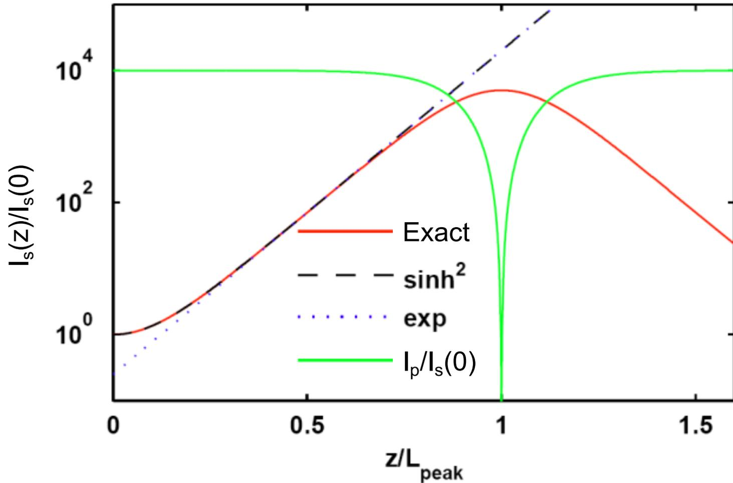
**Fig.** Exact solution for signal gain, plotted together with hyperbolic secant and exponential function solutions, approximate solutions derived by assuming the pump is undepleted. The exact solution for the pump intensity is also shown.
