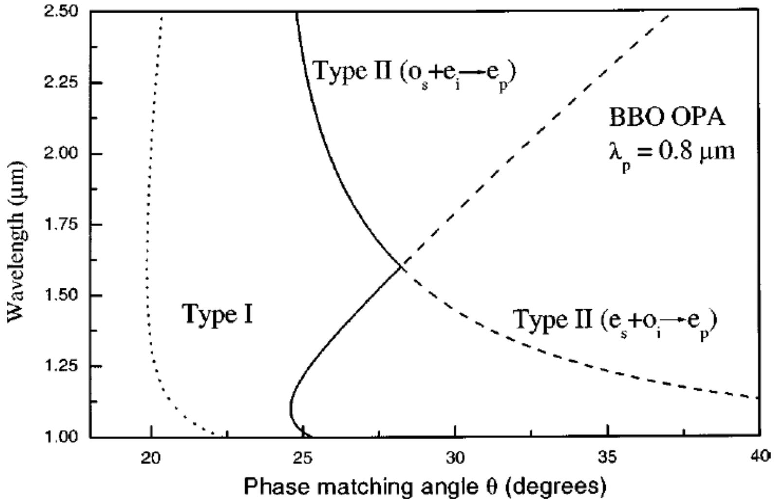
**Fig. 12.28** Angle tuning curves for a BBO OPA at the pump wavelength  $\lambda_p = 0.8 \mu\text{m}$  for type I phase matching (dotted line), type II ( $o_s + e_i \rightarrow e_p$ ) phase matching (solid line), and type II ( $e_s + o_i \rightarrow e_p$ ) phase matching (dashed line).
