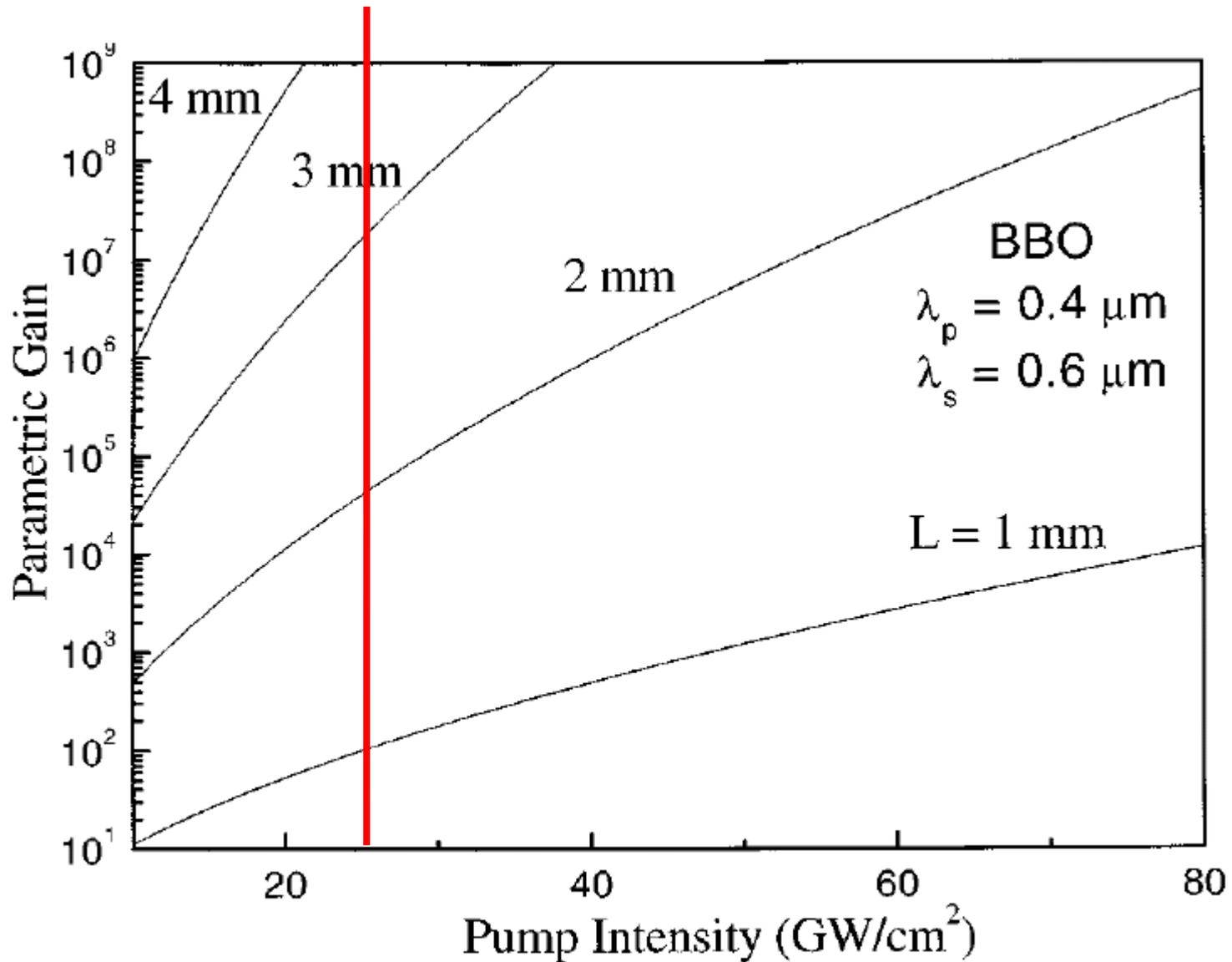
**Fig. 12.25** Parametric gain for an OPA at the pump wavelength  $\lambda_p = 0.4 \mu\text{m}$  and the signal wavelength  $\lambda_s = 0.6 \mu\text{m}$ , using type I phase matching in BBO ( $d_{\text{eff}} = 2 \text{ pm/V}$ ).
