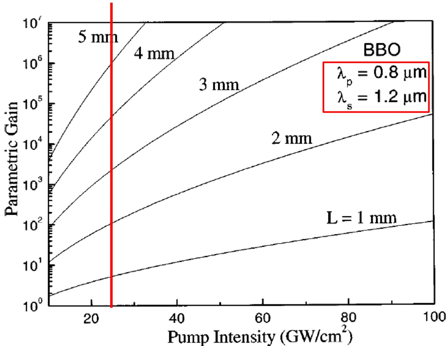
**Fig. 12.24** Parametric gain for an OPA at the pump wavelength  $\lambda_p = 0.8 \mu\text{m}$  and the signal wavelength  $\lambda_s = 1.2 \mu\text{m}$ , using type I phase matching in BBO ( $d_{\text{eff}} = 2 \text{ pm/V}$ ).
