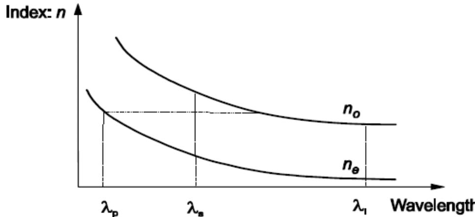
Fig. 12.26 Type I noncritical phase matching.
