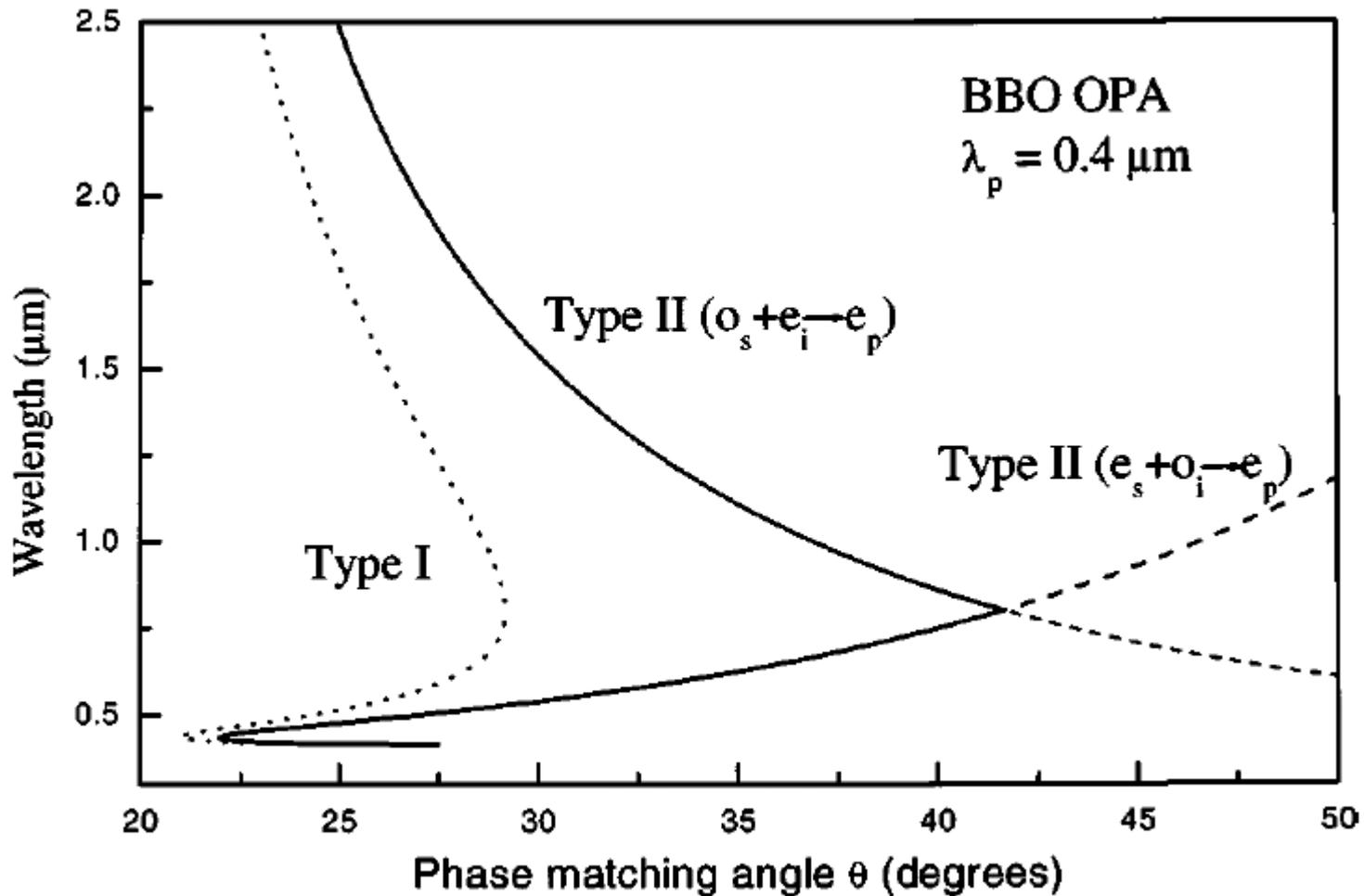
**Fig. 12.28** Angle tuning curves for a BBO OPA at the pump wavelength  $\lambda_p = 0.4 \mu\text{m}$  for type I phase matching (dotted line), type II ( $o_s + e_i \rightarrow e_p$ ) phase matching (solid line), and type II ( $e_s + o_i \rightarrow e_p$ ) phase matching (dashed line).
