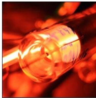
Methan-stabilized HeNe-Laser in a molecular optical clock
