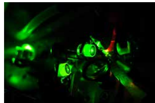
High repetition rate Kerr-Lens Mode-locked Ti:sapphire laser.
