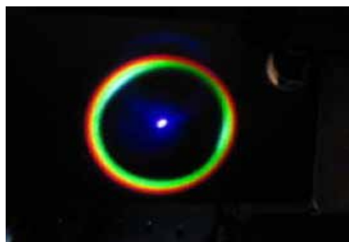
Superfluorescence cone in optical parametric amplifiers.
