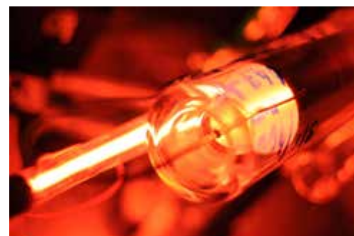
Methane-stabilized HeNe-Laser in a molecular optical clock.
