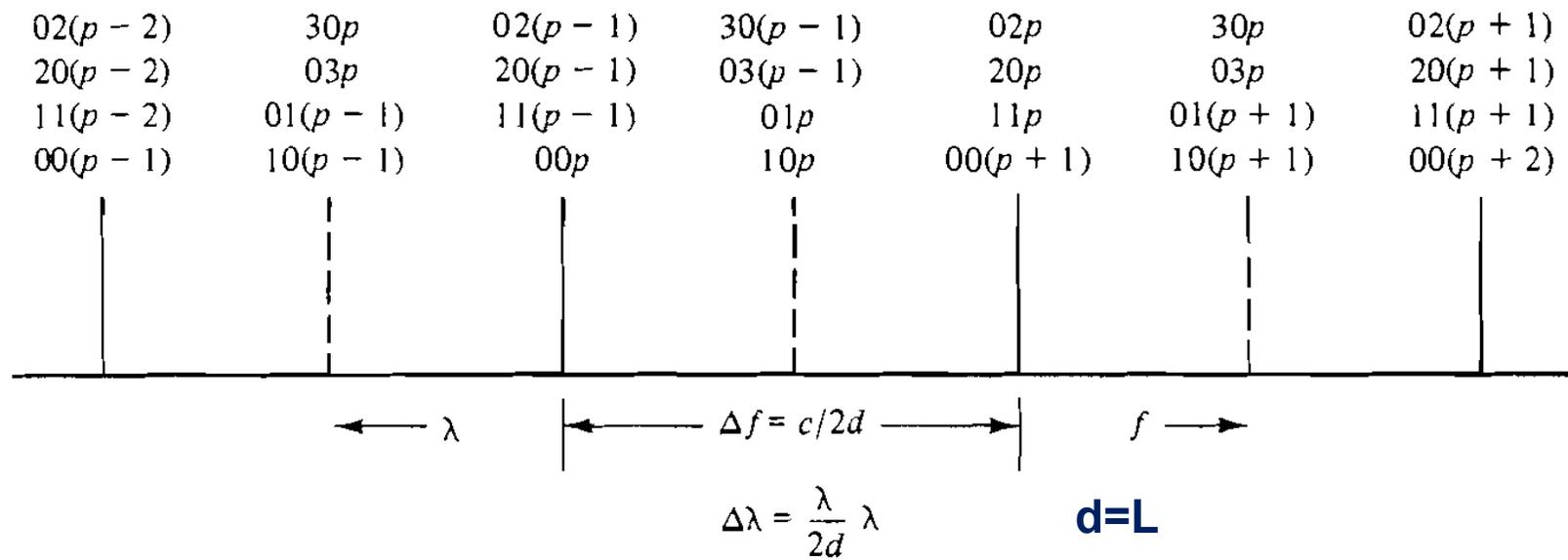
**Figure 2.29:** Resonance frequencies of the confocal Fabry-Perot resonator,
