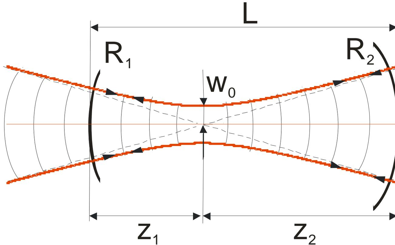
*Figure 2.20: Fabry-Perot Resonator with finite beam size.*
