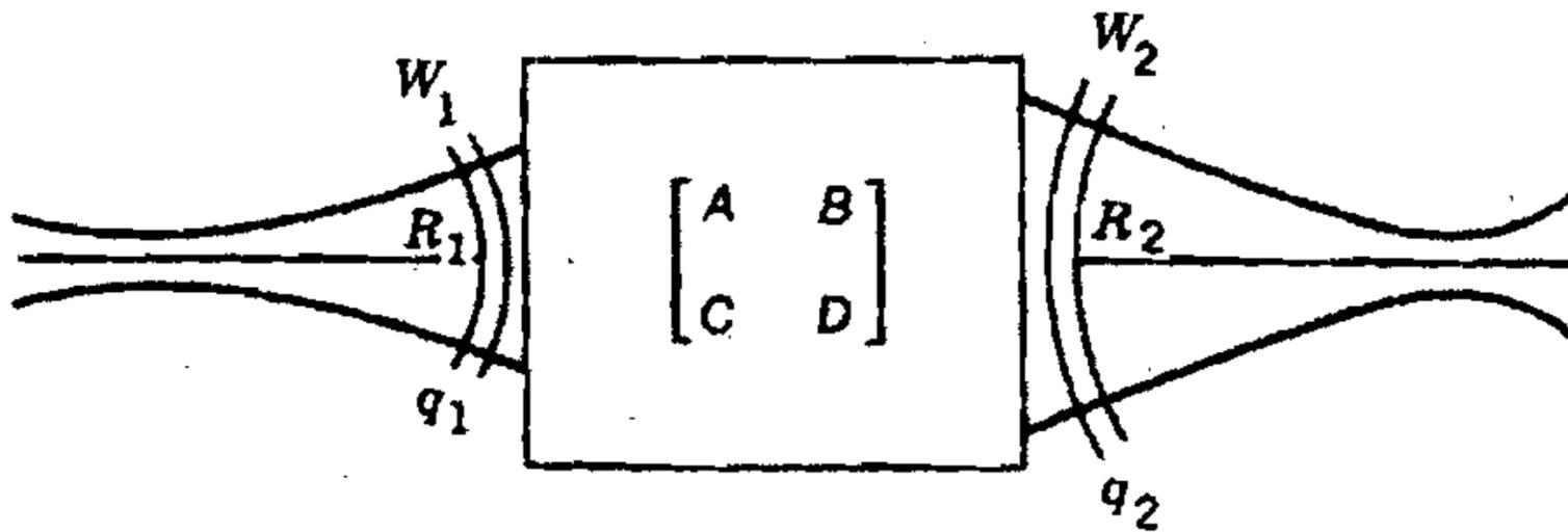
*Figure 2.18: Gaussian beam transformation by ABCD law.*
