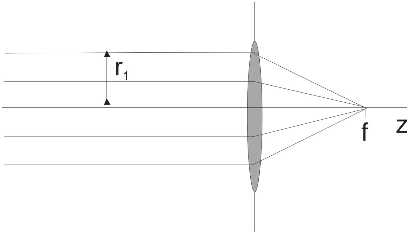
*Figure 2.15:* Imaging of parallel rays through a lens with focal length  $f$
