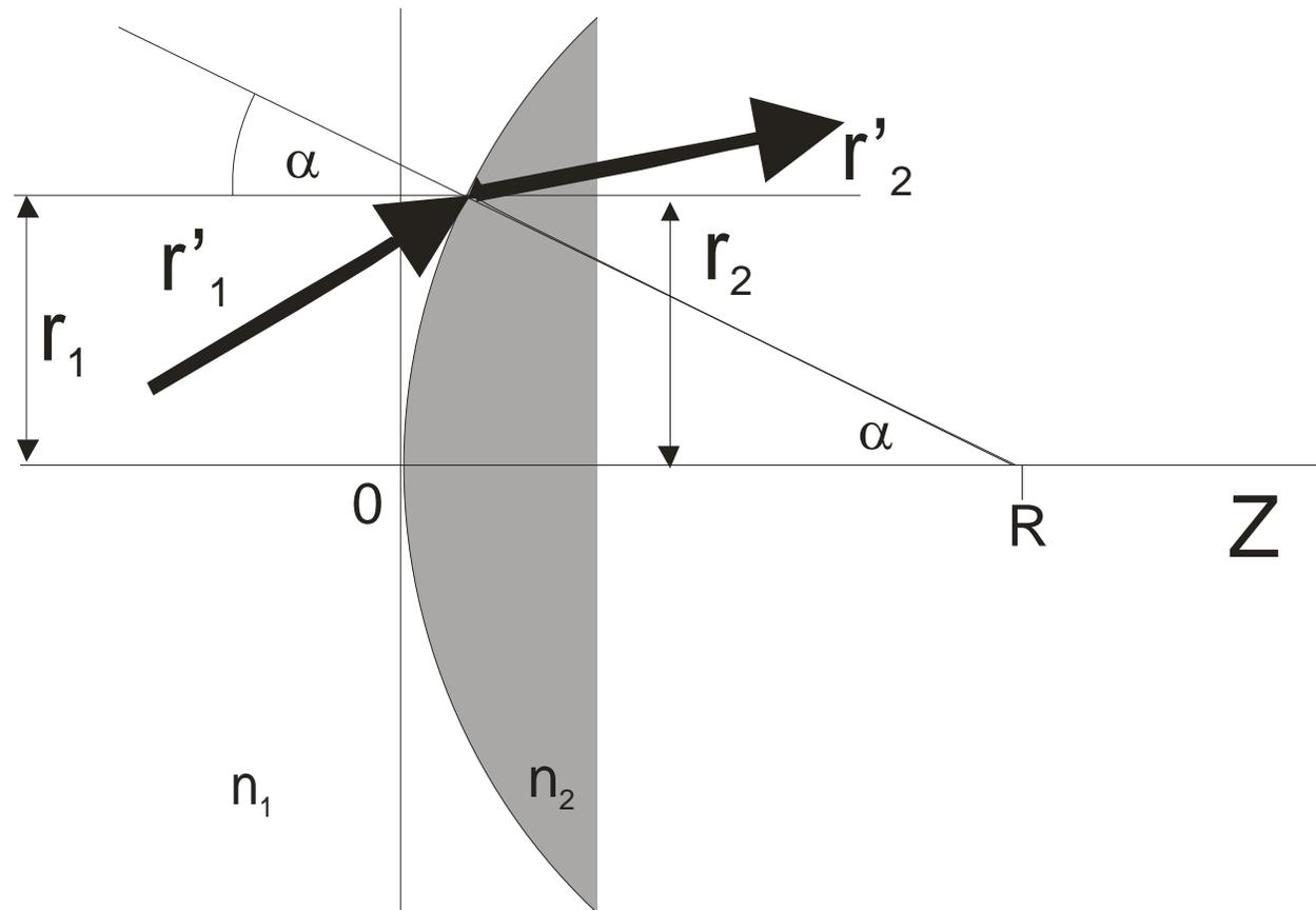
Figure 2.14: Derivation of ABCD-matrix of a thin plano-convex lens.
