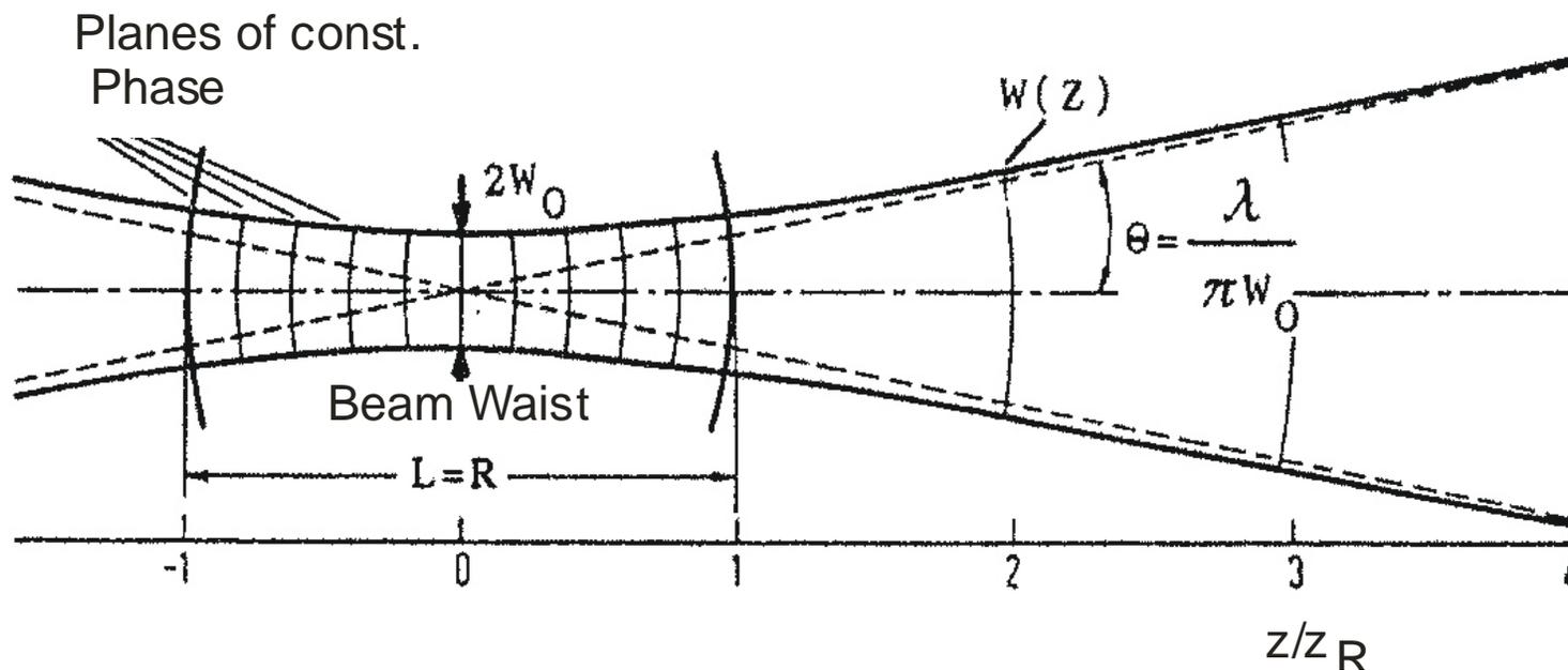
Figure 2.66: Gaussian beam and its characteristics
