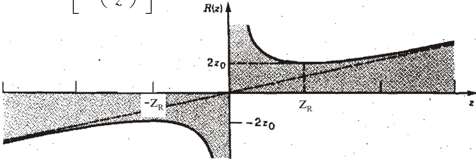
Figure 2.7: Radius of curvature  $R(z)$
