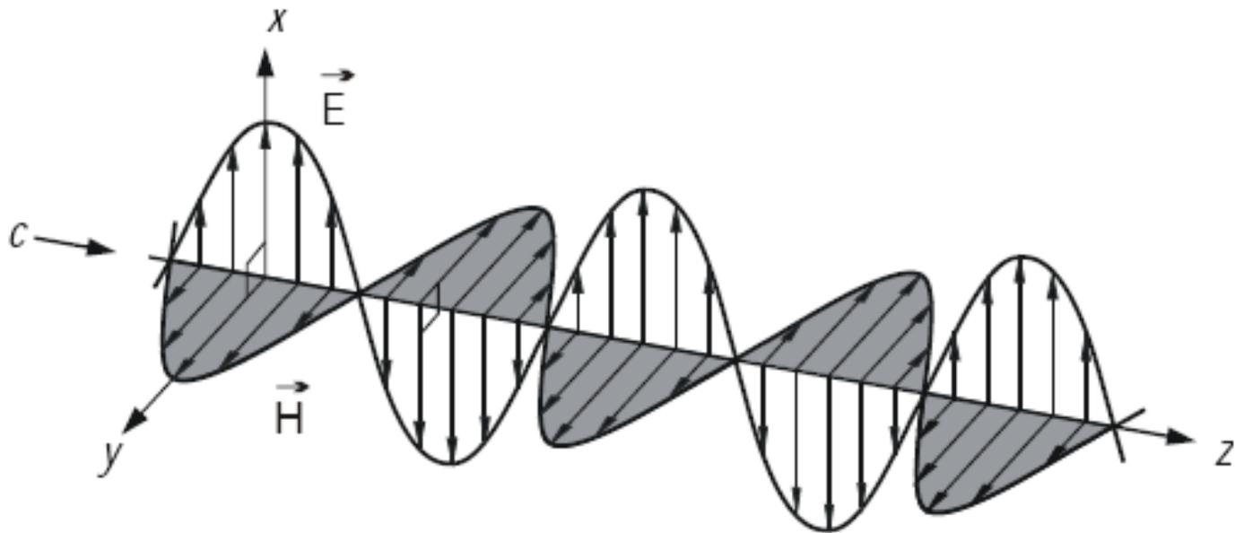
Figure 2.1: Transverse electromagnetic wave (TEM) [6]
