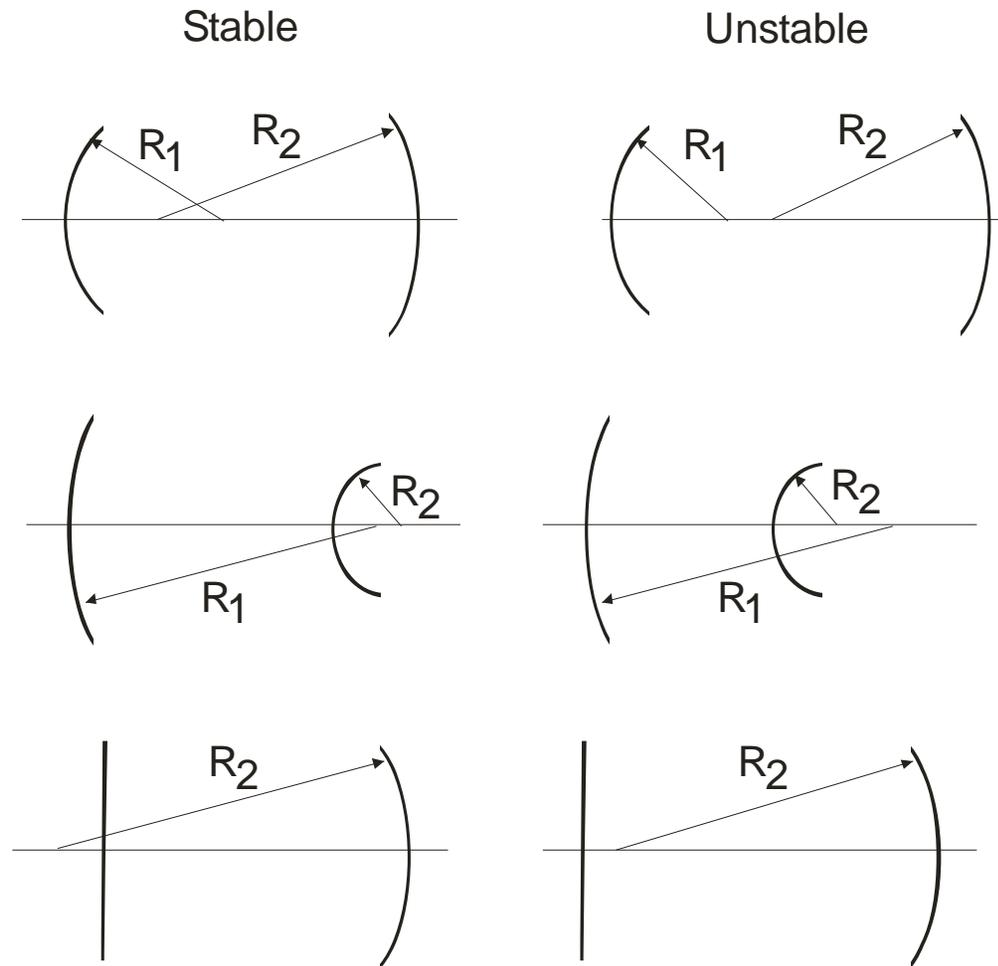
**Figure 2.26: Stable and unstable resonators**
