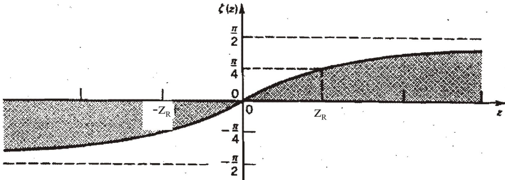
Figure 2.6: Phase delay of Gaussian beam, Guoy-Phase-Shift
