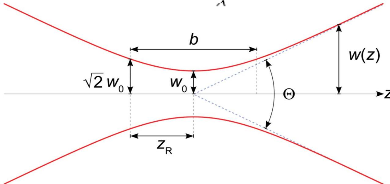
Figure 2.5: Gaussian beam and its characteristics
