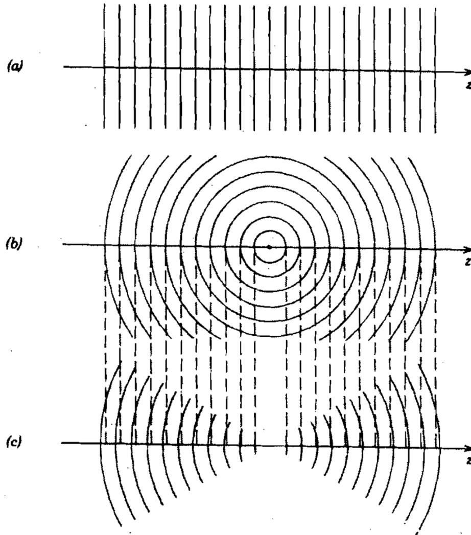
*Figure 2.9:* Wavefronts of (a) a uniform plane wave, (b) a spherical wave; (c) a Gaussian beam.
