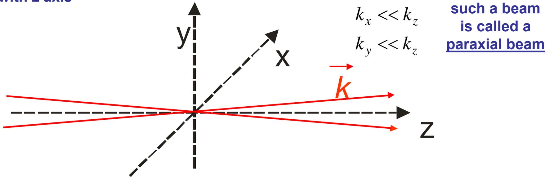
Figure 2.2: Construction of paraxial beam by superimposing many plane waves with a dominant k-component in z-direction
