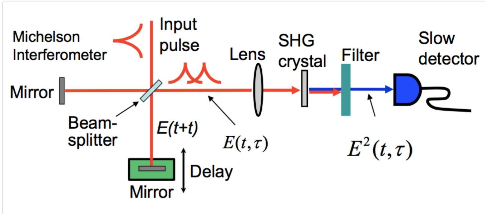
An alternative approach is to use a collinear beam geometry, and allow the autocorrelator signal light to interfere with the SHG from each individual beam
