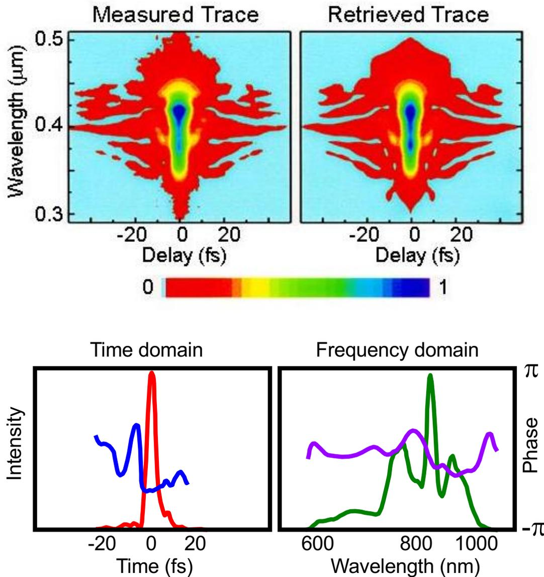
Agreement between the experimental and reconstructed FROG traces provides a nice check on the measurement.
