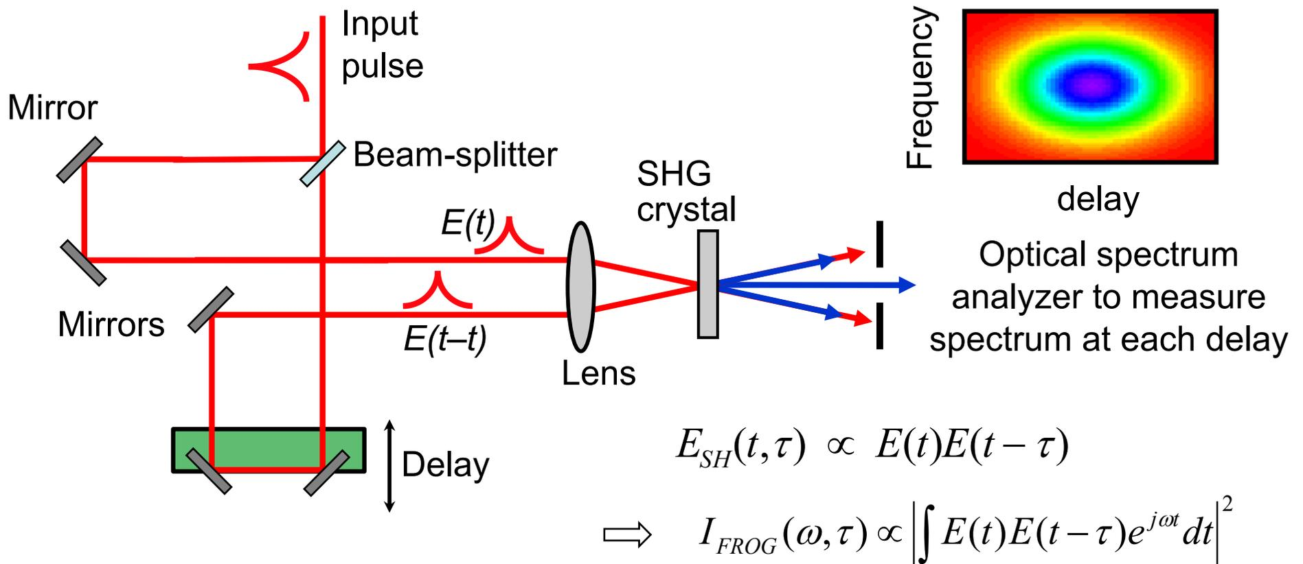
Now we have N X N data points. Iterative algorithm can retrieve both the amplitude and phase of the measured optical pulse.
