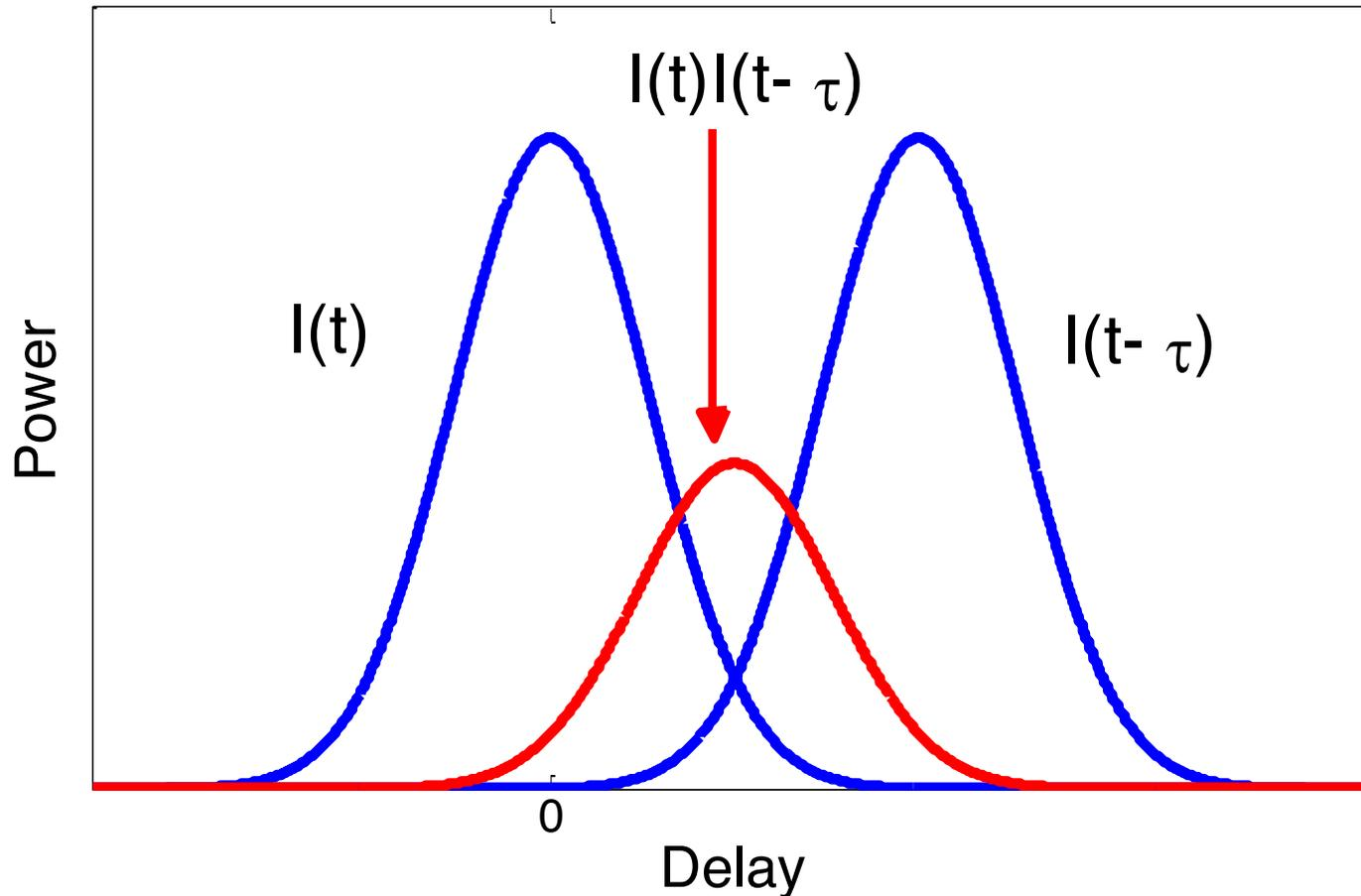
Varying the delay yields varying overlap between the two replicas of the pulse.
