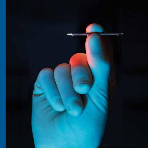
Terahertz accelerator modules fit easily between two fingers.
