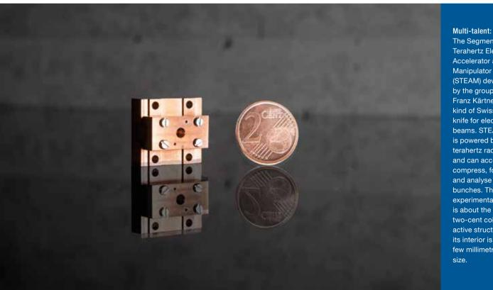
The Segmented Terahertz Electron Accelerator and Manipulator (STEAM) developed by the group of Franz Kärtner is a kind of Swiss Army knife for electron beams. STEAM is powered by terahertz radiation and can accelerate, compress, focus and analyse electron bunches. The experimental device is about the size of a two-cent coin. The active structure in its interior is just a few millimetres in size.
